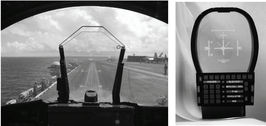
Figure 17-1. Examples of head-up displays (HUDs): (left) a HUD in a fighter cockpit and (right) a HUD designed for aircraft simulation (Rockwell Collins).
