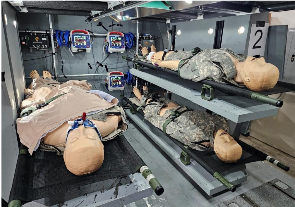
Figure 2. Three-patient configuration patient layout used during data collection (Patient one is on the left, patient two is on the top right, and patient three is on the bottom right).
