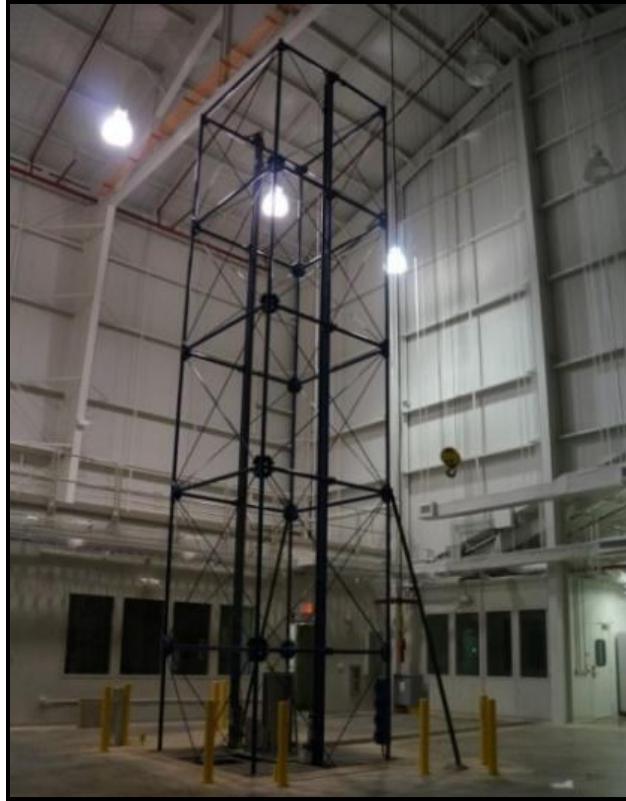
Figure 4. The USAARL HYGE™ (Kittanning, PA) VAT was used to produce the vertical crash pulse for this study.
