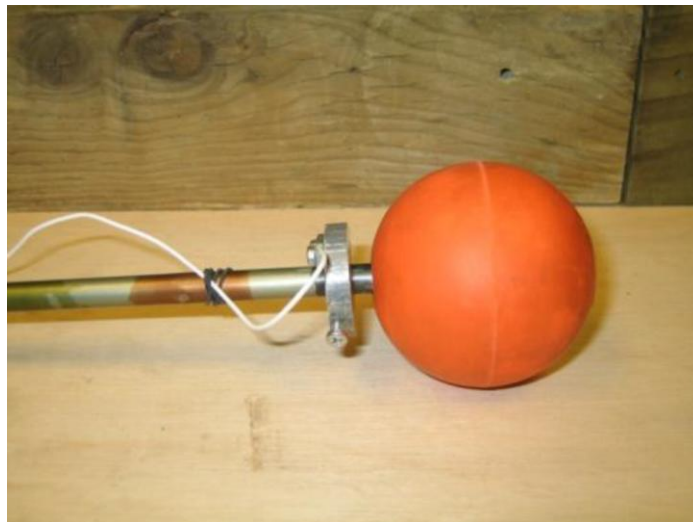
Figure 11. The ball shaft impactor was designed by using a lacrosse ball attached to an aluminum shaft. The accelerometer was attached to the impactor via an aluminum disc that was mounted to the shaft directly behind the ball. Figure reproduced with permission from Dau (2012).
