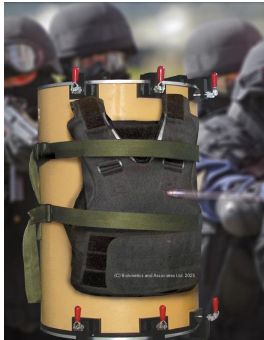
Figure 10. The first generation BTTR had a cylindrical shape based on average chest breadth and approximated curvature for correct armor fit. Figure reproduced with permission from Biokinetics and Associates, Ltd.
