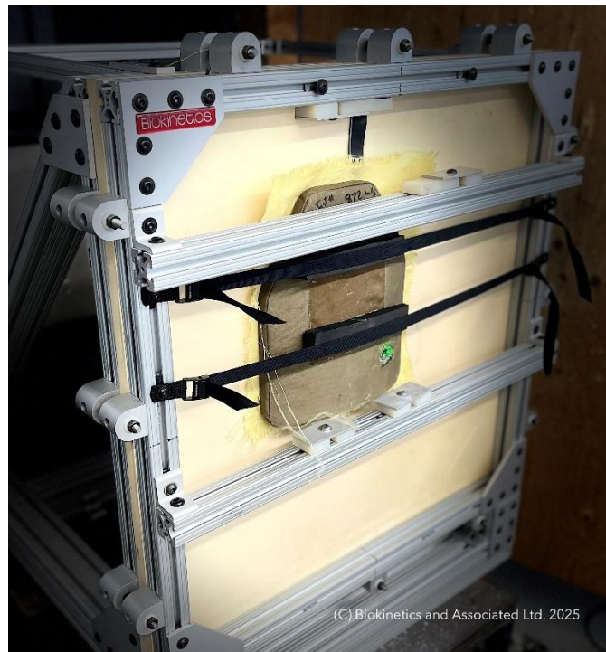
Figure 16. The f-BTTR system membrane setup and 3D BFD measurement system was designed to allow for 3D transient measurements. Figure reproduced with permission from Biokinetics and Associates, Ltd.
