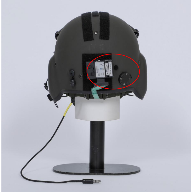
Figure 6. Depiction of EEG receiver mounted on back of helmet.
