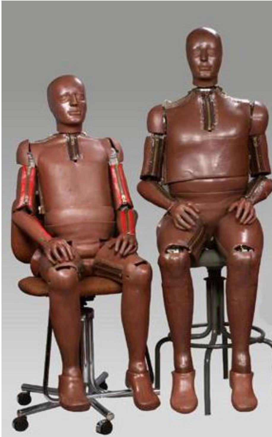
Figure A12. ADAM reproduced from Thomas (2014) with permission of Christopher Perry, Biodynamics Section, Wright Patterson Air Force Base. Instrumentation includes linear and angular accelerometers, neck/lumbar load cells, and angular potentiometers. These are no longer available for procurement.
