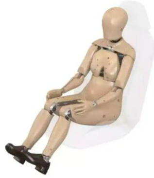
Figure A4. The Test Device for Human Occupant Restraint (THOR) 5F ATD reproduced with permission from Humanetics Group (2023a).
