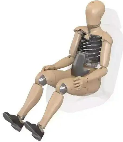
Figure A3. The THOR-50M ATD reproduced with permission from Humanetics Group (2023b).
