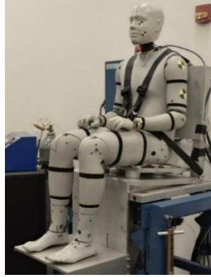
Figure A16. WIAMan Technology Demonstrator seated in the vertical loading condition reproduced with permission from David Weyland (U.S. Army DEVCOM Ground Vehicle Systems Center).
