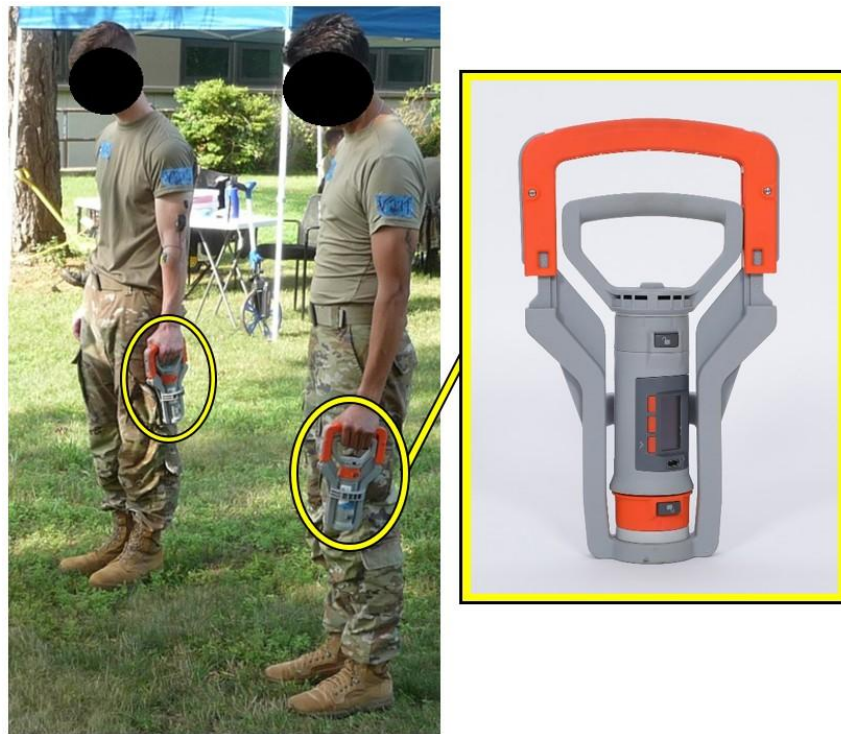
Figure 5. VALD DynaMo Plus dynamometers (right) were used to record grip strength before and after each carry condition. One of the litter teams is pictured (left) conducting the grip strength test before a carry condition.
