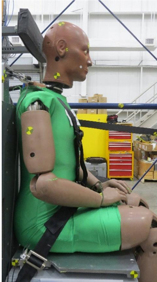
Figure 3. The FAA-HIII ATD, configured with the FOCUS headform, was positioned in a 90-90-90 rigid seating system.
