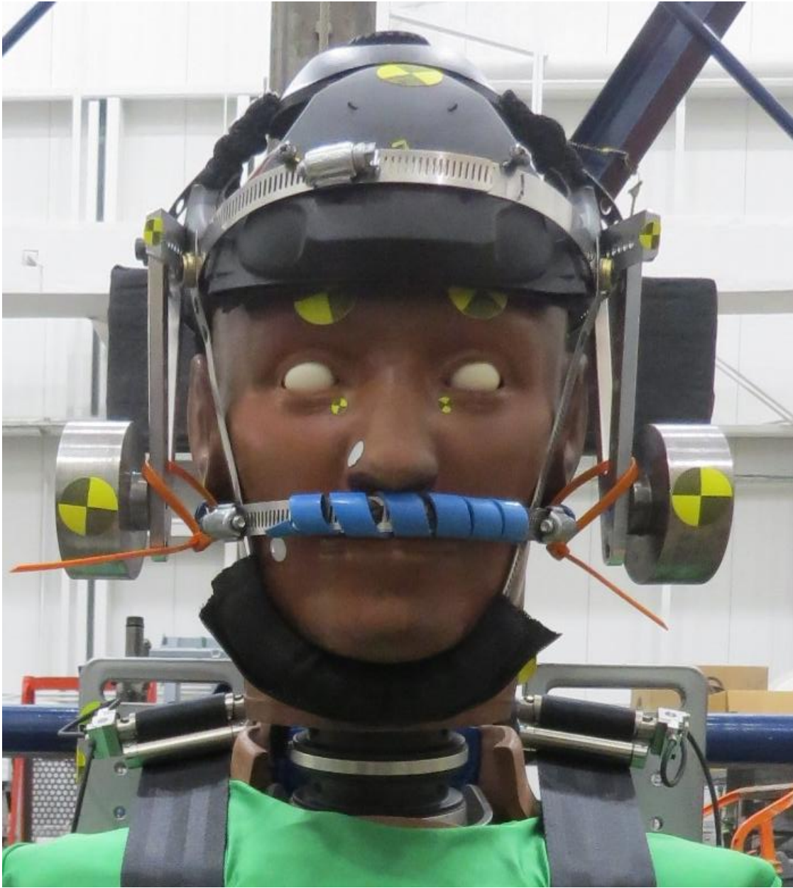
Figure 7. The research team used zip ties (orange) fastened between the triangular bracket and the nose hose clamp to minimize movement of the triangular bracket and mass relative to the FOCUS headform during vertical acceleration.
