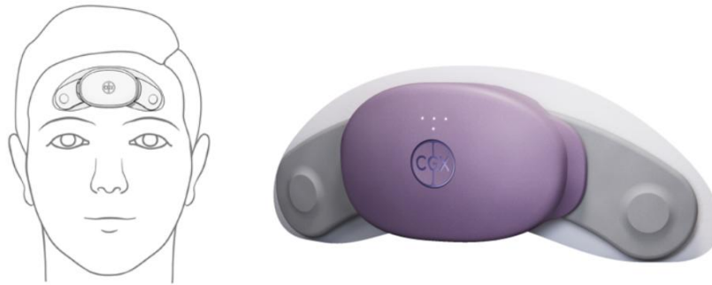
Figure 1. Image of CGX EEG Patch location demonstrated on forehead.
