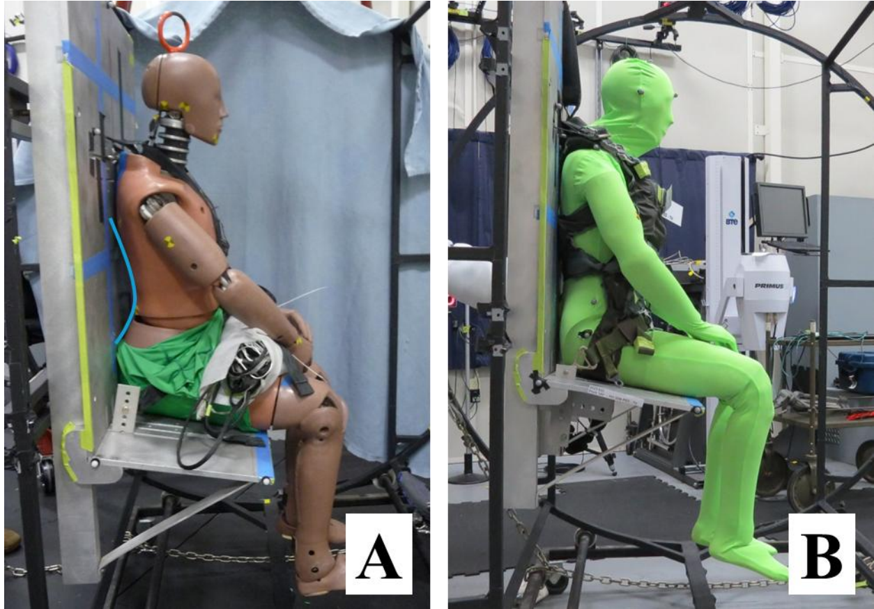
Figure 3. The FAA-HIII-50M (A) and HIII-50M-P (B) were tested to determine their compatibility with the seat assembly. The molded pelvis of the FAA-HIII-50M made positioning difficult and left a gap between the seatback and the ATD back (indicated by the blue line [A]). The articulating pelvis of the HIII-50M-P allowed for better positioning of an occupant with most of the back in contact with the seatback.
