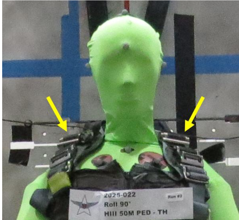
Figure 6. The TH straps were instrumented with load cells (yellow arrows), where possible.
