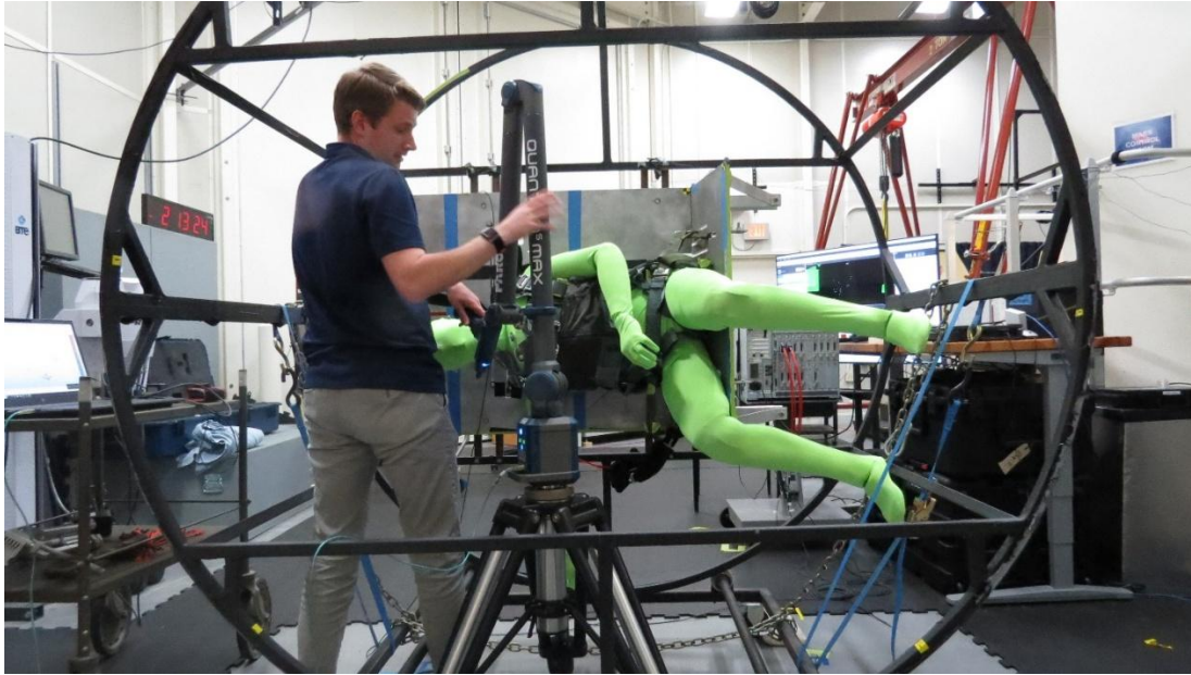
Figure 14. The FaroArm® Quantum Max had to be positioned inside of the inversion wheel to complete measurements. Here, the test fixture is in the 90-degree roll configuration.
