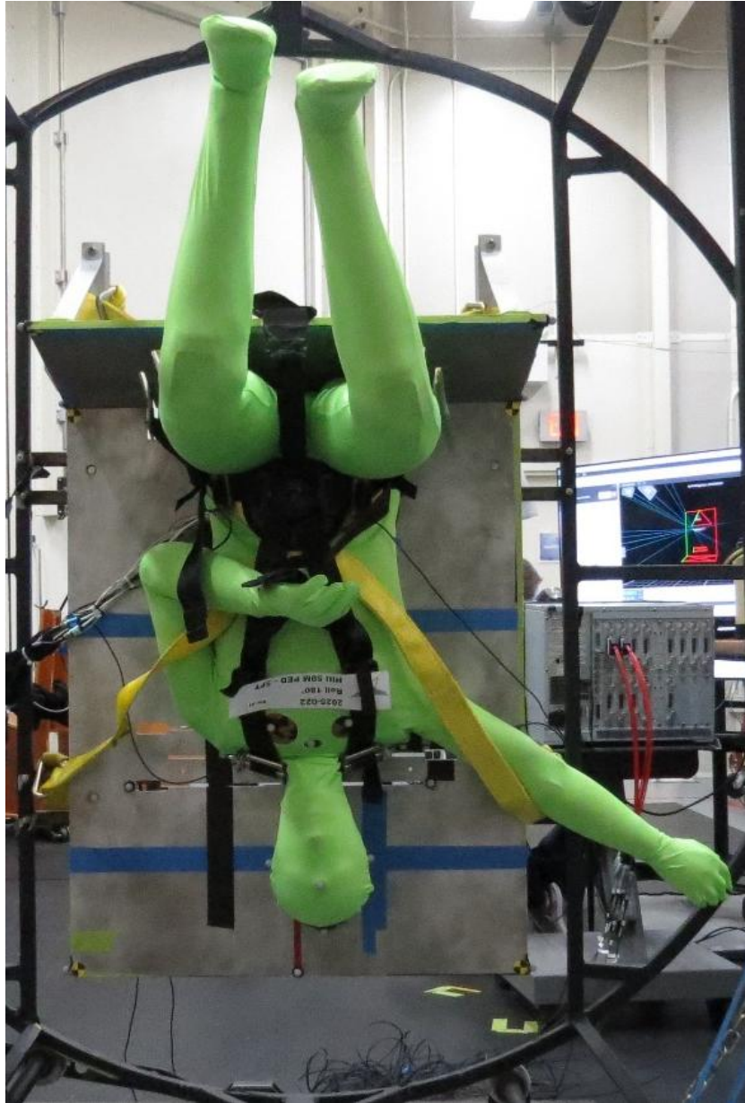
Figure 9. The ATD was further secured with yellow safety straps to prevent it from completely falling out of the seat assembly during restraint release. This figure demonstrates the pre-release 180° roll position.
