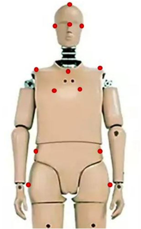
Figure 7. Retroreflective markers were placed on the ATD to capture displacement during the rotation of the inversion wheel.
