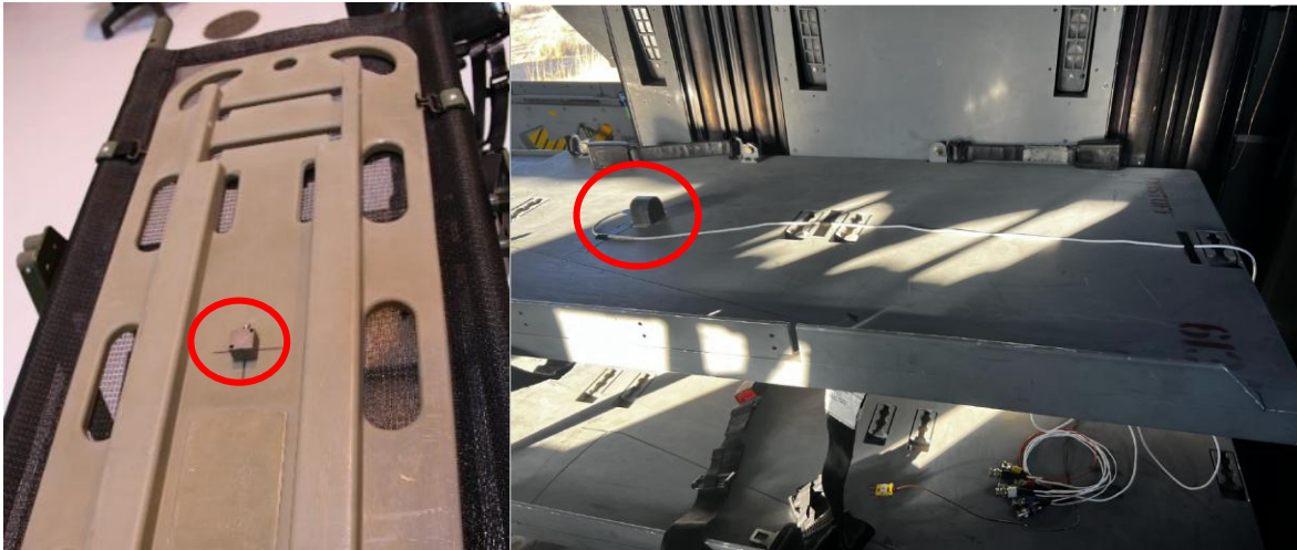
Figure 6. Spine board 6DOF sensor location (left), and litter pan sensor location (right).
