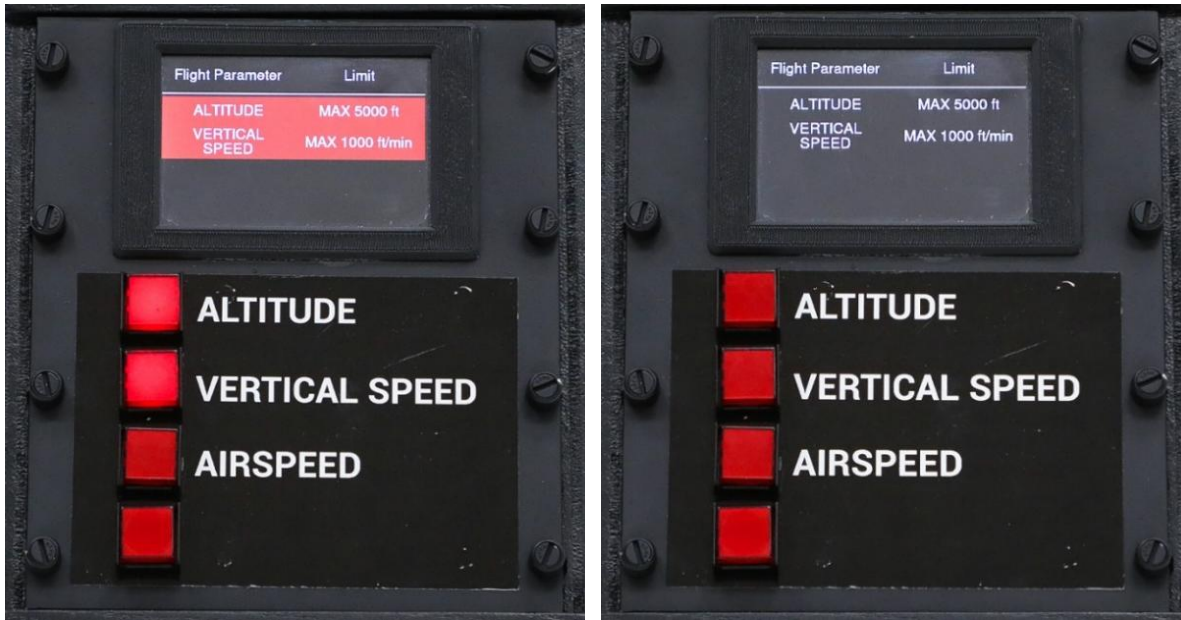
Figure 2. The pilot aid displaying restrictions (left, active restrictions; right, acknowledged restrictions).
