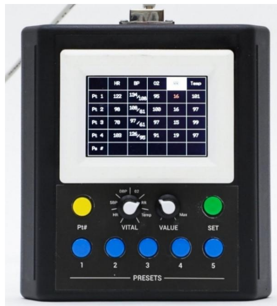
Figure 5. The physical prototype of the patient emulator is shown.
