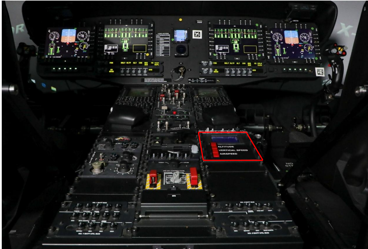
Figure 1. The STEPS pilot aid (outlined in red) installed within CAPT-E VCS simulator.
