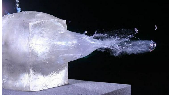
Figure 16. A 9 mm bullet was photographed while traversing ballistic gelatin. The image shows a bullet traversing the gelatine block, entering on the left and exiting on the right. There is a large temporary cavity seen in the block for the entire bullet path and material is exuded on the right following the bullet shear (Groover & Boor, 2014).
