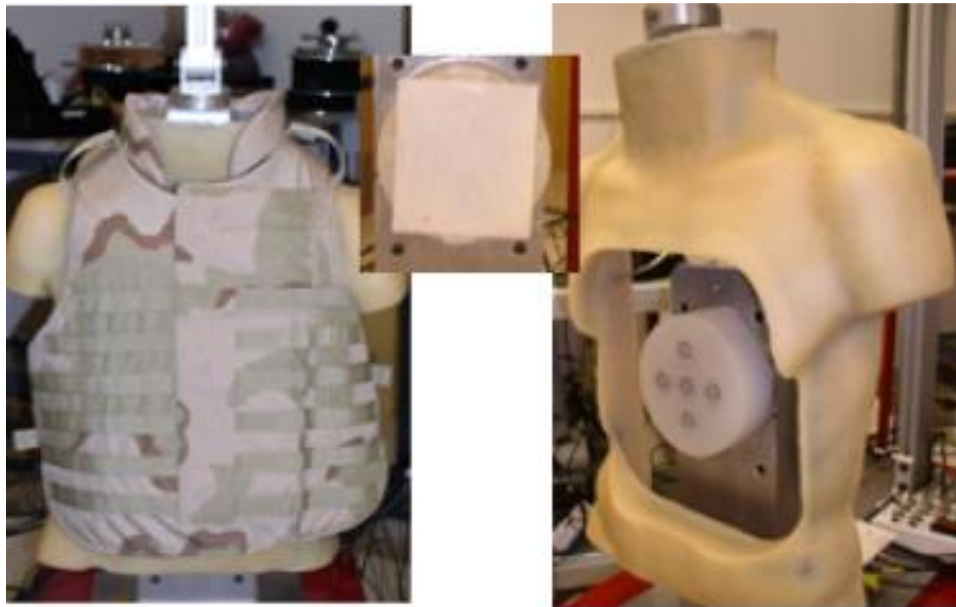
Figure 24. The ATM with mounted body armor (left) is shown without body armor (right) to reveal the response element within the torso. The ATM instrumented response element with padding is shown in the center. Reproduced from Leggieri (2010) with permission from The National Academies Press.
