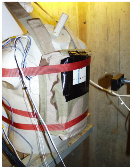
Figure 26. The AUSMAN thorax is shown with body armor in place prior to testing. Note the protrusion from the neck is a simulated trachea. Use of this trachea and the Hybrid III neck mount would need to be coordinated with a custom neck and lower neck load cell.
